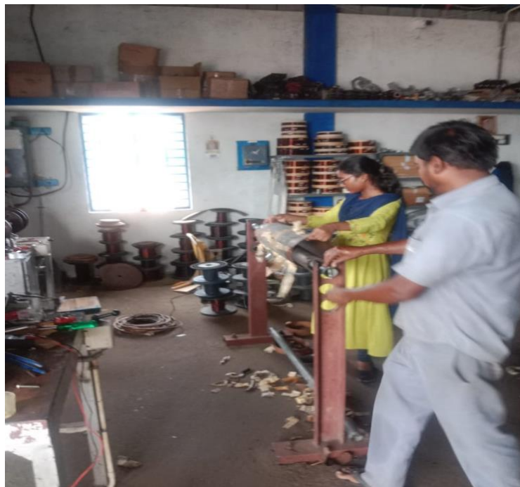
FIG.1.22: RECOILING OF LV WINDING
