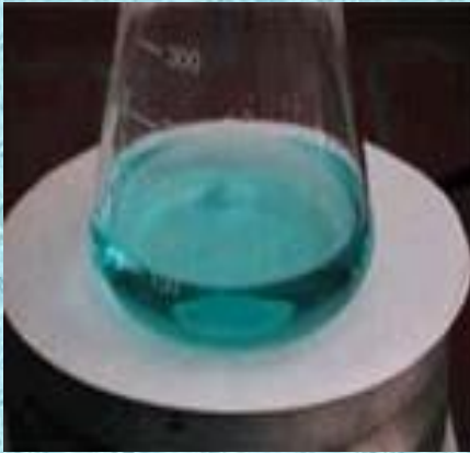
Luminol and peroxidase before adding \text{H}_2\text{O}_2
